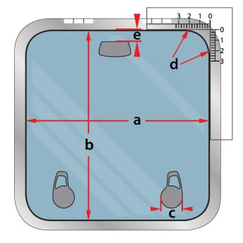
а The width across the lens including the caulk line where the caulk line meets the frame.
